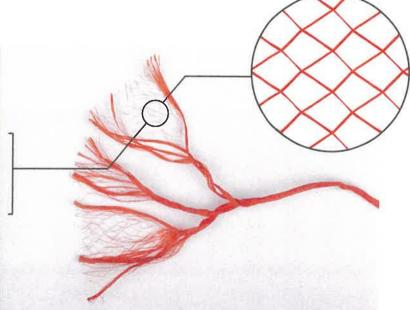
Thor twines are manufactured on a state-of-the-art EVOTAPE extruder and feature our unique TiteLoc fibrillation technology. TiteLoc increases knot holding capability compared to standard polypropylene twines of the same runnage (m/kg).
